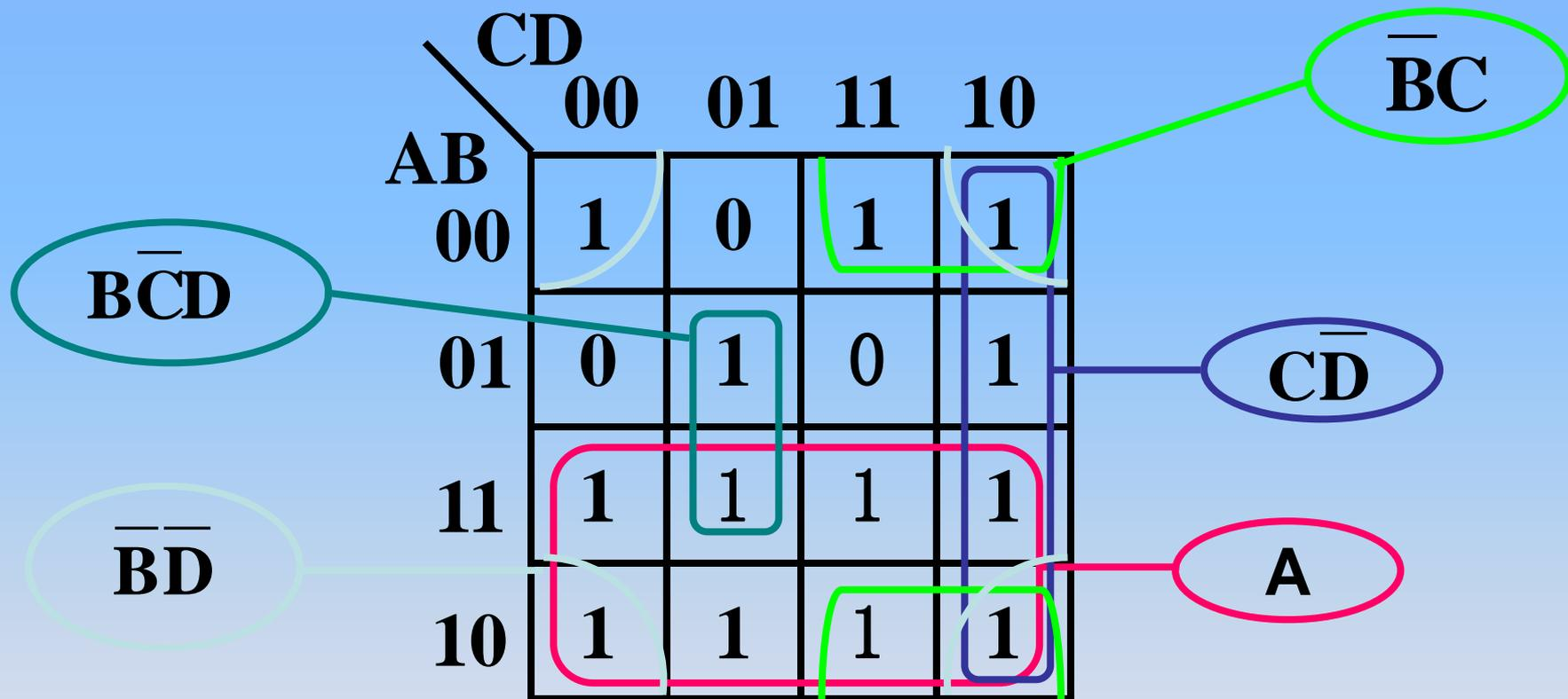
$$F = A + C\bar{D} + \bar{B}C + \bar{B}\bar{D} + \bar{B}C\bar{D}$$
