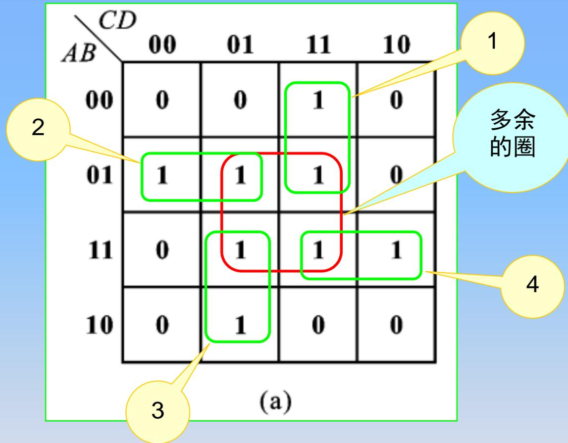
$$Y = \bar{A}CD + \bar{A}B\bar{C} + A\bar{C}D + ABC$$
